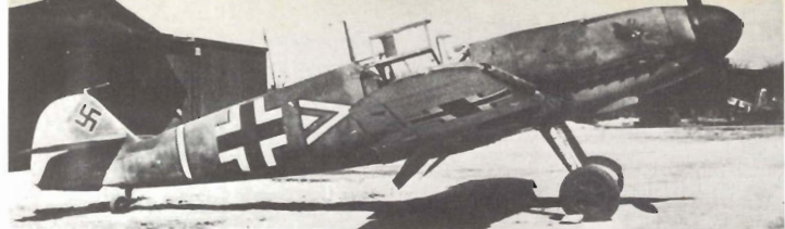
Bf 109F flown by the adjutant of III./JG 2 "Richtofen", Caen, France 1941. Note the upper surface camouflage has been carried over and slightly under the leading edge of the wing. (via M. C. Windrow)
