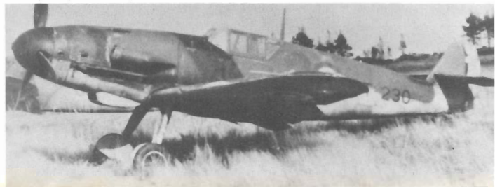
Below: MT-230 in the olive green and black camouflage, unit unknown, probably HLeLv 31. Note the darker areas where the earlier target insignia has been overpainted. (via Eino Ritaranta)
